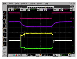
Figure 9. Signal repetition in case different nodes coincidentally transmit on both branches. Blue – TxD signal of the node on bus1 (delayed with an RC constant); magenta – TxD signal of the node on bus 2; yellow and green – bus voltage on bus1.
