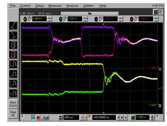
Figure 10. Signal repetition in case different nodes coincidentally transmit on both branches. Yellow and green – bus voltage on bus1; blue and magenta – bus voltage on bus2. Overall view and zoom on the transition dominant->recessive.
