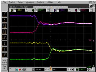
Figure 8. Signal repetition from CAN bus 2 (blue+ magenta) to CAN bus 1 (yellow + green) in case only one node transmits on bus1. Zooms to both signal transitions
