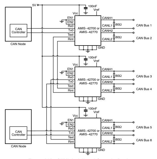
Figure 5. Adding CAN Nodes in Network Connection Board
