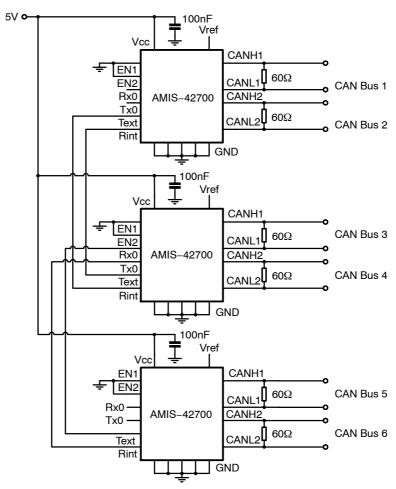
Figure 3. CAN Bus Network Connection Board
