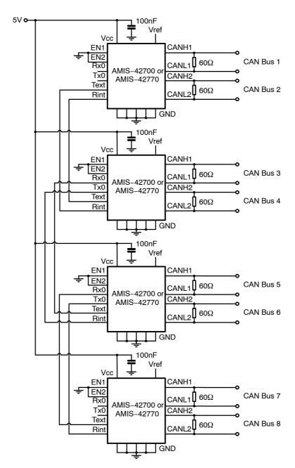
Figure 4. 8 CAN Bus Network
