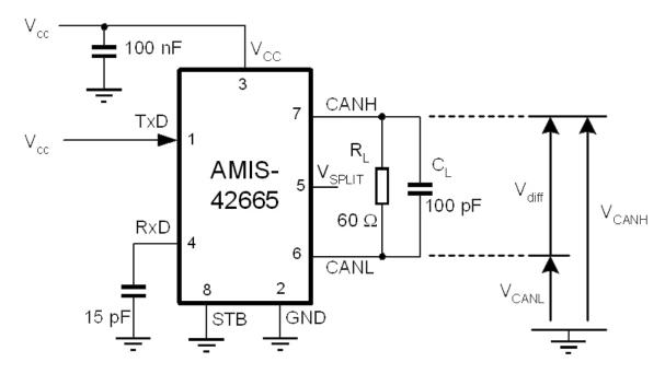
Figure 1. Set-up V<sub>CANH</sub> and V<sub>CANL</sub>
