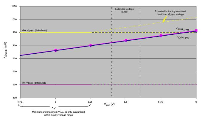
Figure 6. AMIS-42665 Differential Receiver High Threshold Voltage
