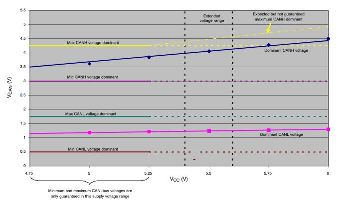
Figure 4. AMIS-42665 CAN-Bus Voltages
