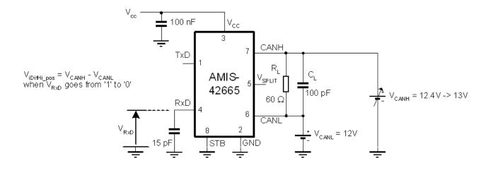
Figure 2. Differential Receiver High Threshold Voltage for CMV = +12 V
