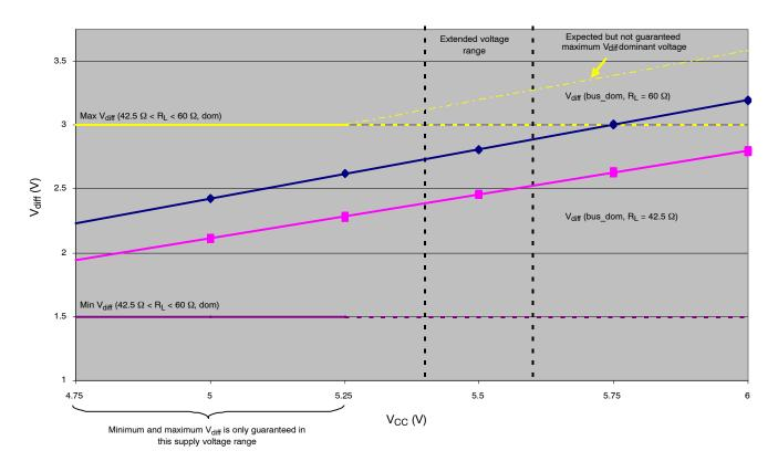
Figure 5. AMIS-42665 Dominant Differential Bus Output Voltage
