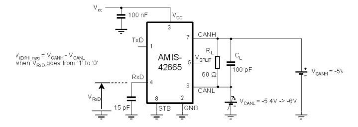
Figure 3. Differential Receiver High Threshold Voltage for CMV = -5 V
