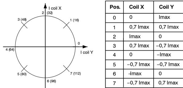
**Figure 3. Motor Current for Half Step Mode**
