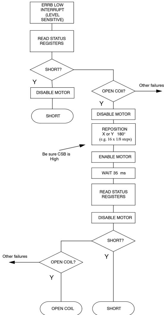
Figure 4. 100% Coverage Short Detection to GND
