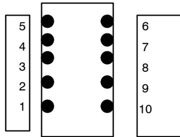
Figure 3. Bobbin Pinout - Bottom View
