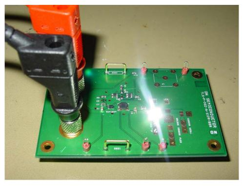
Figure 10. Is NCP1529 Torch Application Demonstration Board
