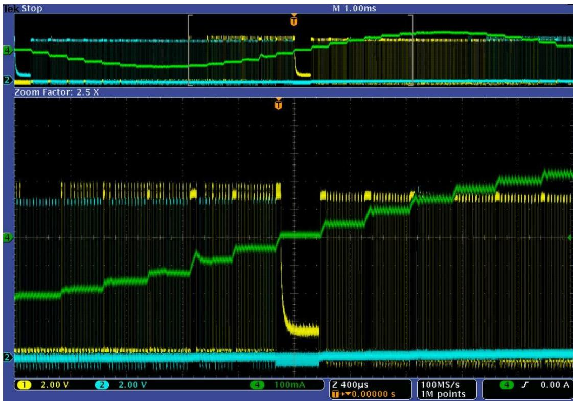
Figure 28. Oscilloscope Plot of Zero Current Crossing
