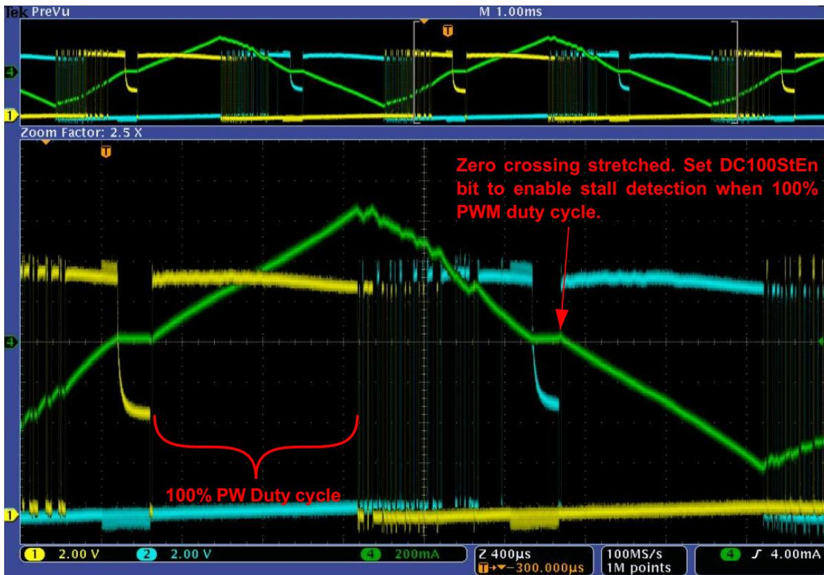
Figure 26. Oscilloscope Plot of 100% PWM Duty-Cycle
