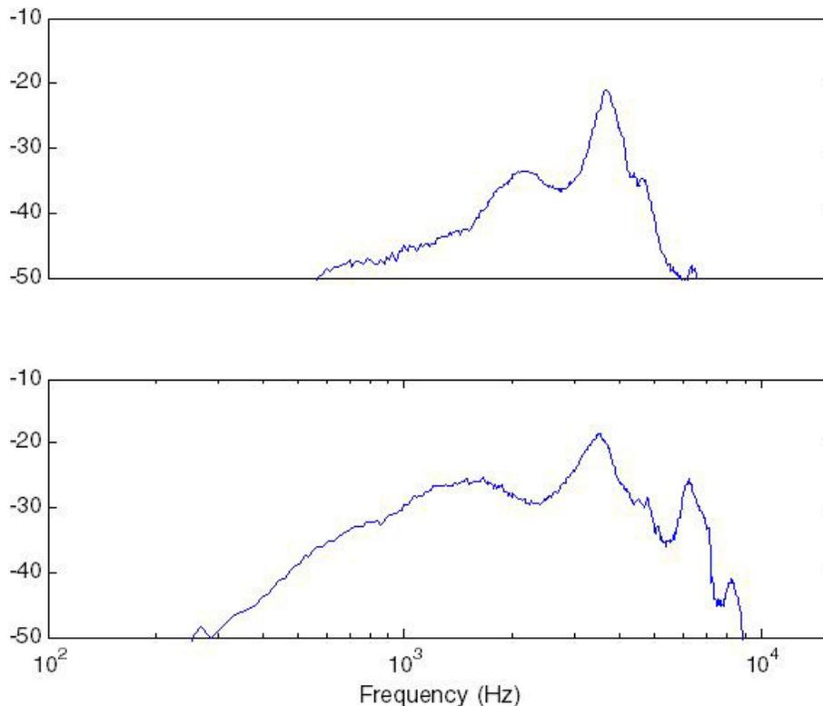
**Figure 7. Frequency response for the two ITE hearing aids shown in Figure 6. Response shown in the top graph has a sharper response peak and will likely result in less ASG compared to the response shown in the bottom graph.**
