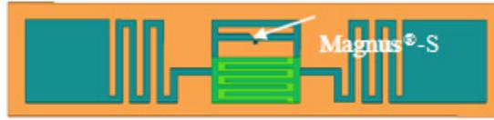
Figure 3. A Capacitance-Based Battery Free Wireless Moisture Sensor
