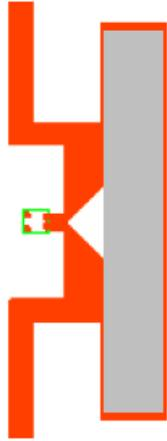
Figure 2. Inductive Loop with Metal Patch
