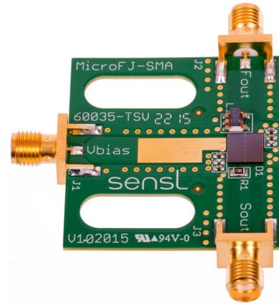
Figure 1. The onsemi 6 mm SMA board (MicroFJ-SMA-60035)
