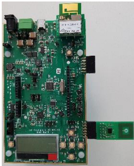
Figure 10. NFC Shield Attached to the IDK Baseboard
