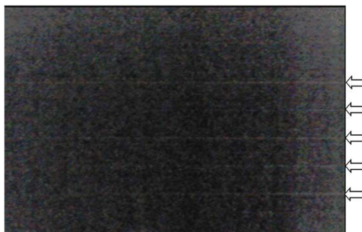
Figure 1. Row Noise at Low Light Condition
