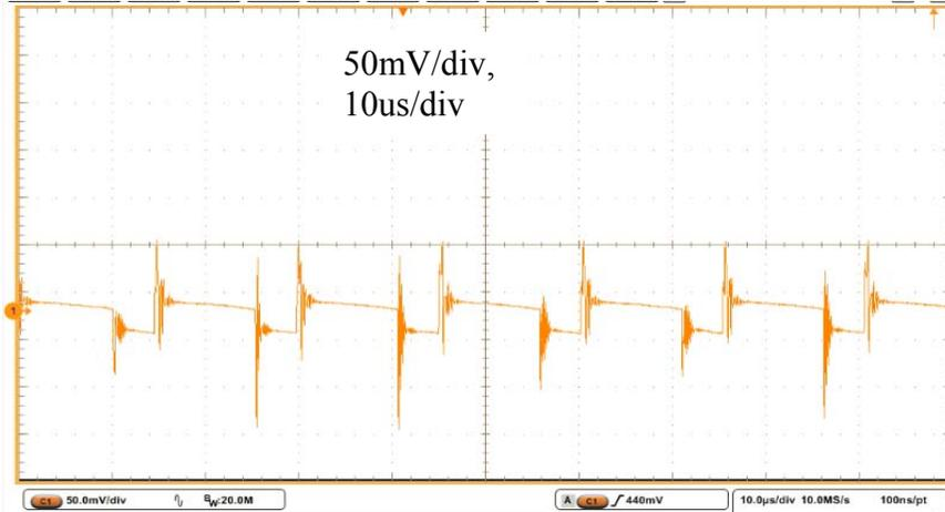
**MOSFET Drain Voltage (120 Vac Input)**
