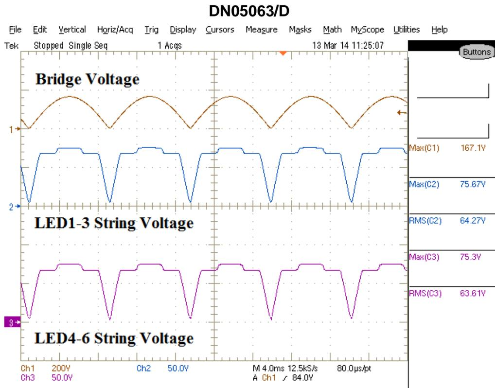
Figure 7 – The LED forward voltage is identical at all times for all LEDs. When the LED voltage is not 0 V, the LEDs are on. Given an LED  $V_f$  of 72 V, the LEDs are on about 72% of the time. The two voltage levels coincide with the parallel/series stages of the driver—as current increases through the LEDs, the voltage increases slightly as well due to series resistance.
