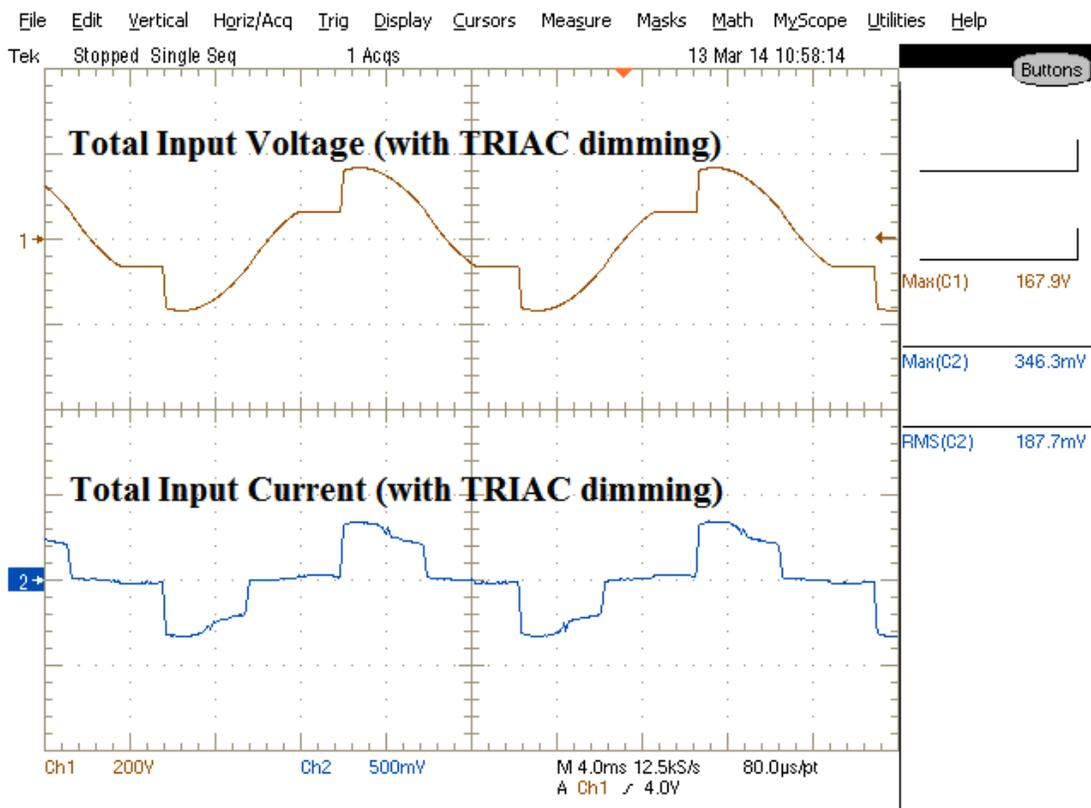
Figure 10 – The circuit receives no input current when the TRIAC is off, and the current is normal when the TRIAC is on.
