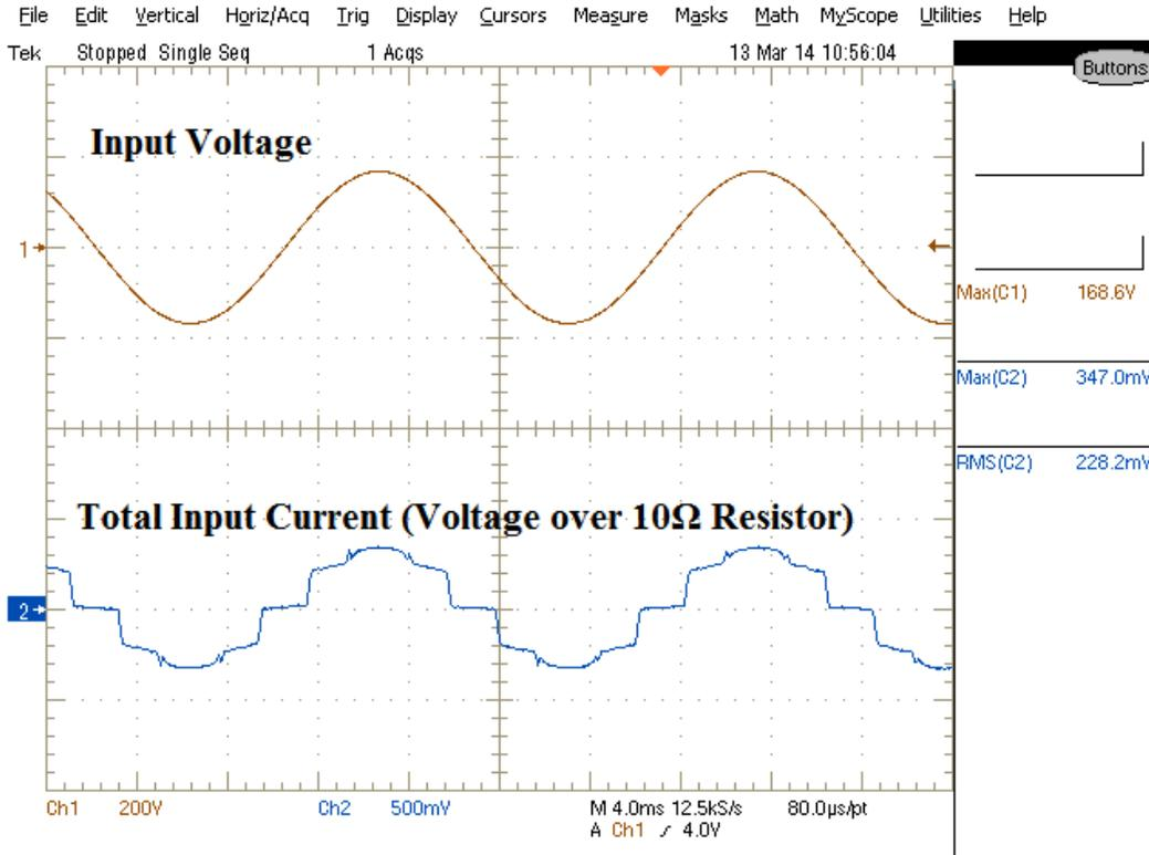
Figure 5 – The total input current follows the voltage waveform very closely, yielding outstanding power factor and THD performance.
