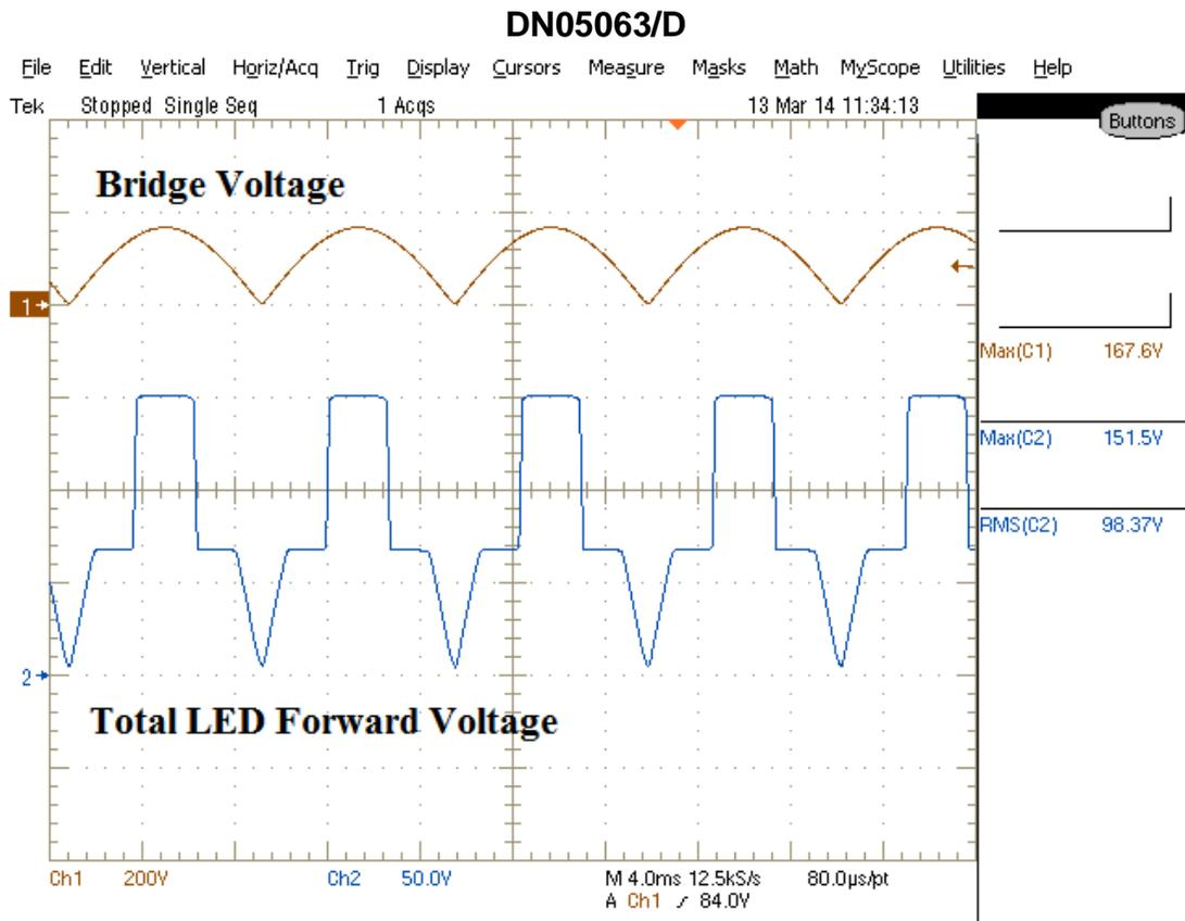
Figure 9 – This capture shows the “total” LED voltage, seen from the CCR cathode to rectified ground. The two levels indicate the LED configurations—the high level is the series mode, and the lower level is the parallel mode.
