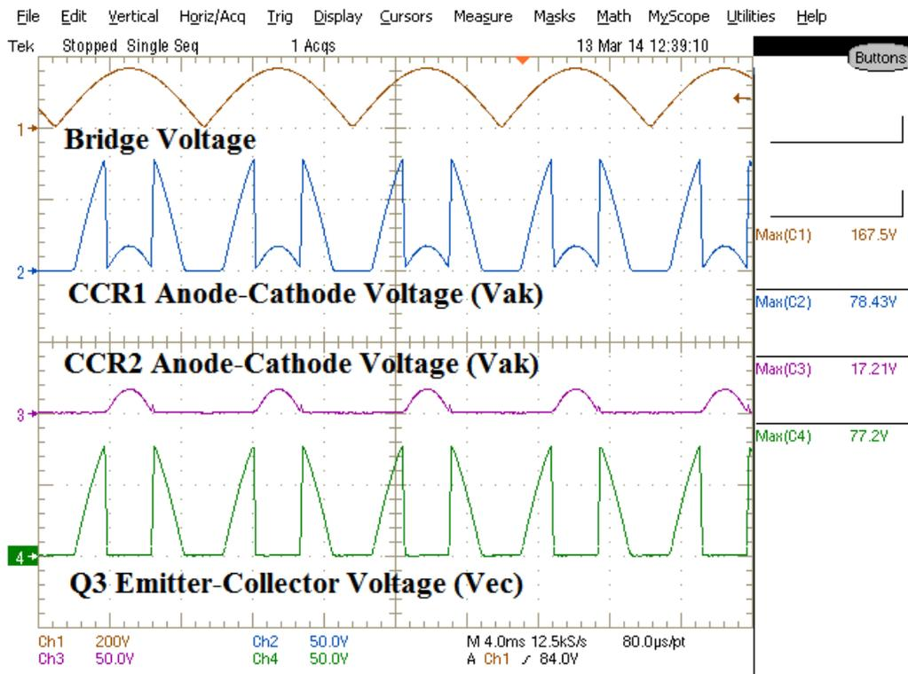
Figure 8 – The CCR1  $V_{ak}$  demonstrates the different stages of the LED configurations. Q3 blocks CCR3 from conducting only until the highest bridge voltages. Q3 and CCR2 are in parallel with CCR1, thus the sum of Q3 and CC2 voltages always equal CCR1.
