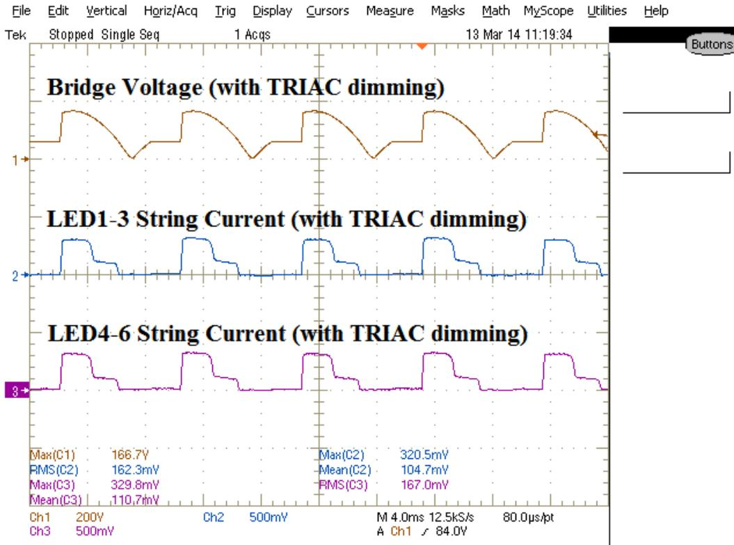
Figure 11 – LED current waveforms are unaffected when the TRIAC is on, and the LEDs shut off perfectly when the TRIAC is off.
