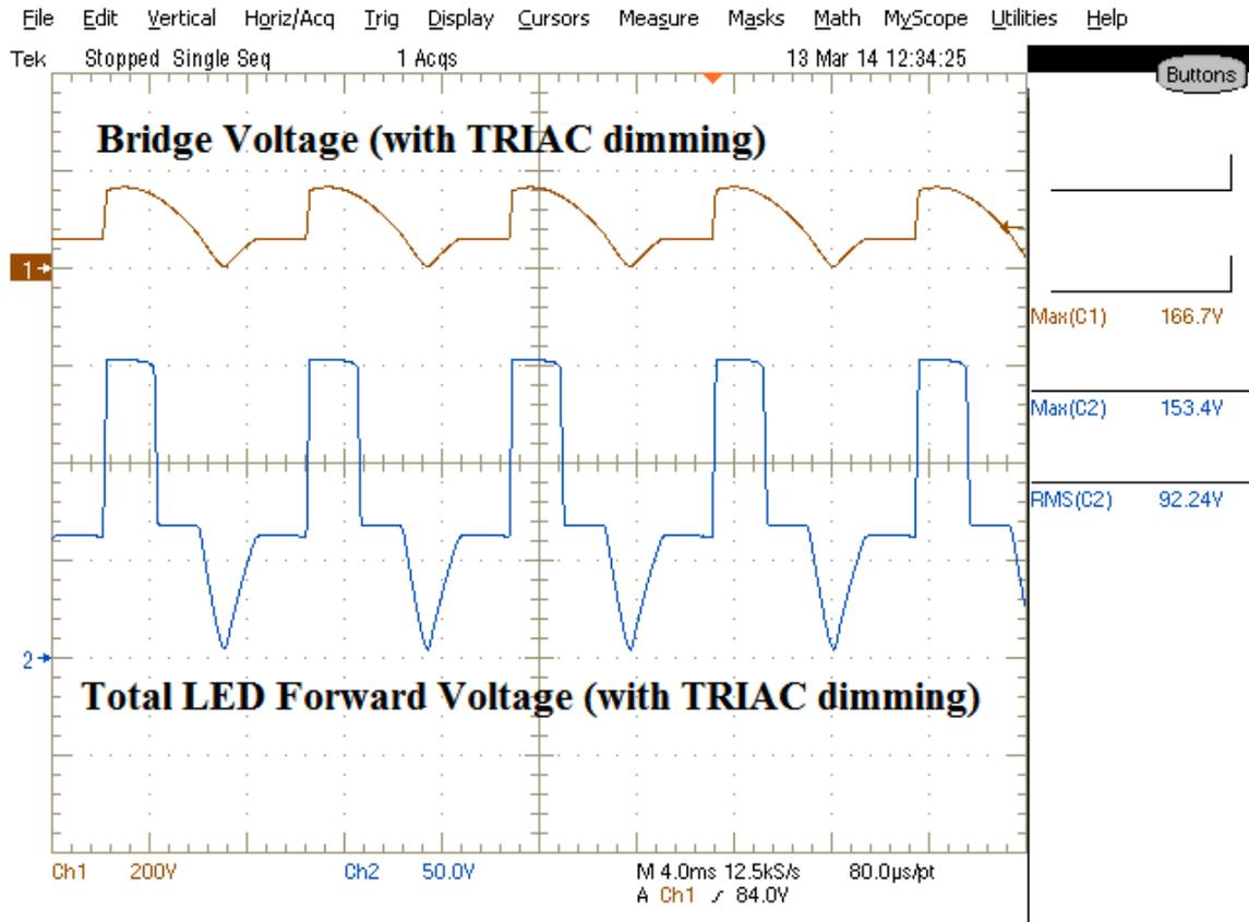
Figure 13 – This capture shows the total LED voltage, showing the configuration of the LED strings during TRIAC dimming. The driver continues to function and switch normally even in the presence of a dimmer.
