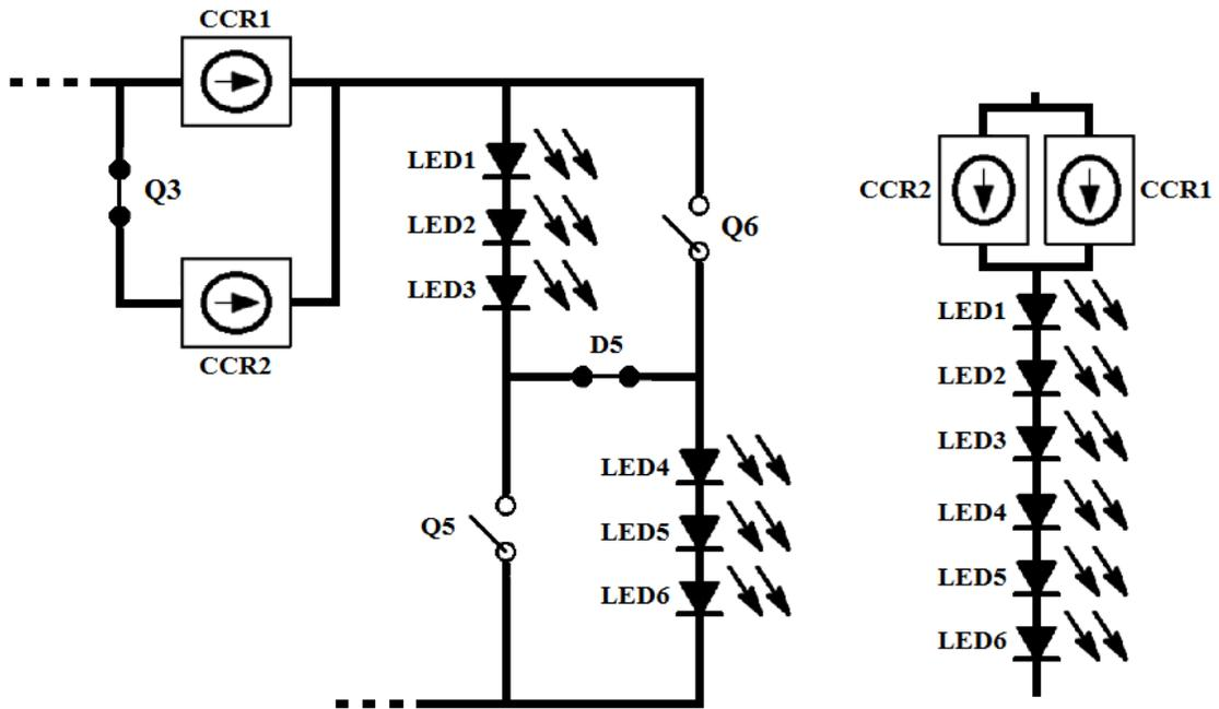
Figure 3 – Stage 2/Series configuration of LEDs. Transistors Q5 and Q6 are now open, and the D5 routing diode connects the two LED strings. The driver is in this state above 158 V.
