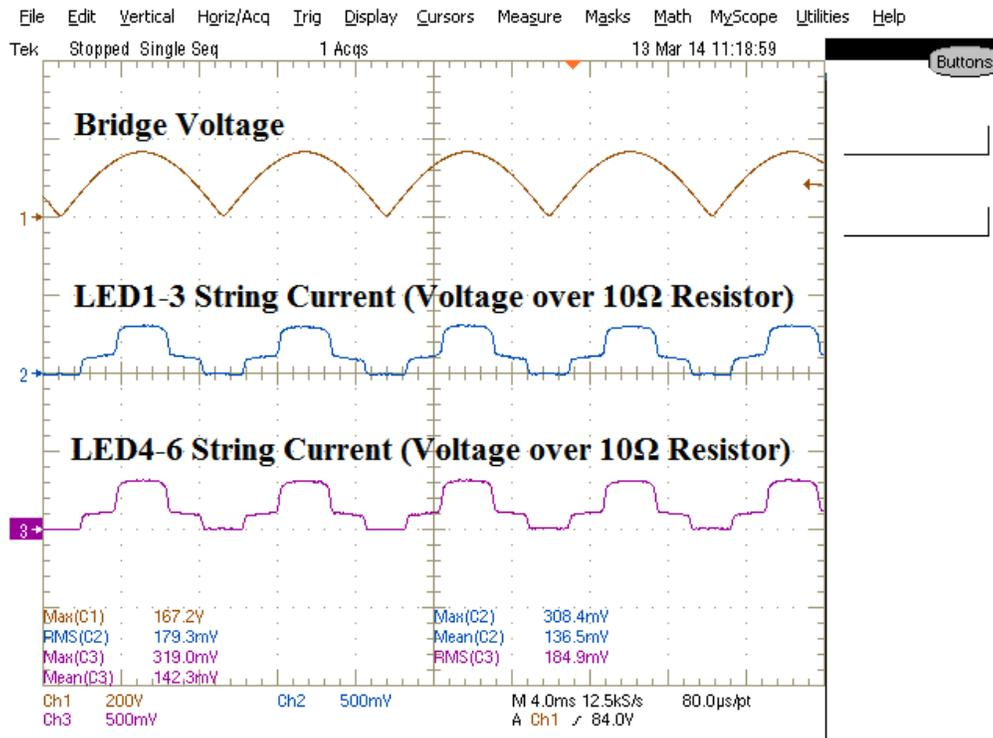
Figure 6 – LED current through each of the LED strings. Note the current waveforms are nearly identical, as well as the two distinct levels of current, coinciding with the two LED configurations.
