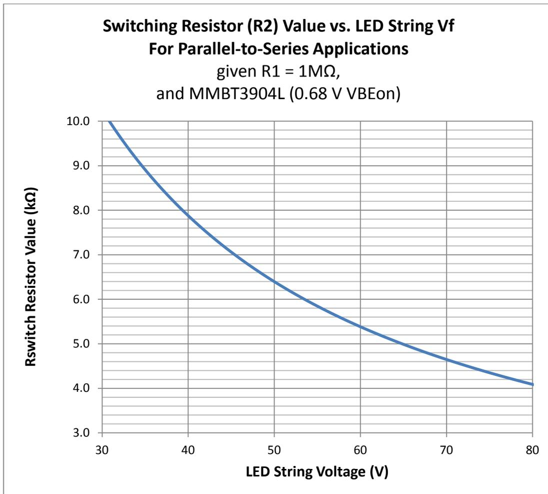
Figure 14 – This graph shows the required R2 resistor value for optimal switching of the LEDs. These values are derived from Equation 1, to serve as a general ballpark for designing with different LEDs.
