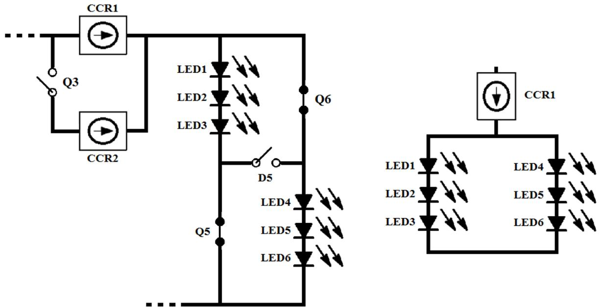
Figure 2 – Stage 1/Parallel configuration of LEDs, showing behavior of switching circuitry. Transistors Q5 and Q6 are on, which reverse biases D5. The LEDs are then in parallel below the CCR. The driver is in this state at bridge voltages below 158 V.
