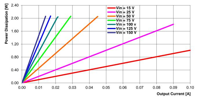
Figure 6. Power Dissipation vs. Output Current
