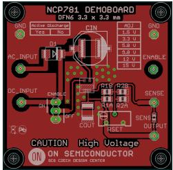
PCB Top Side 1771 mm<sup>2</sup> total Cu area, 1552 mm<sup>2</sup> GND Cu area
