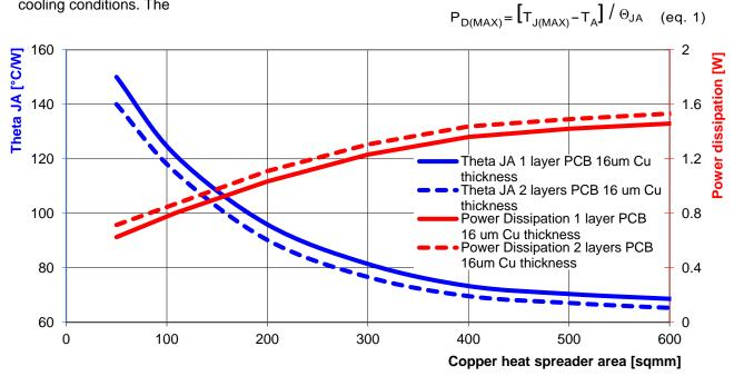
Figure 10. Maximum Power Dissipation & ThetaJA vs. Copper Area
