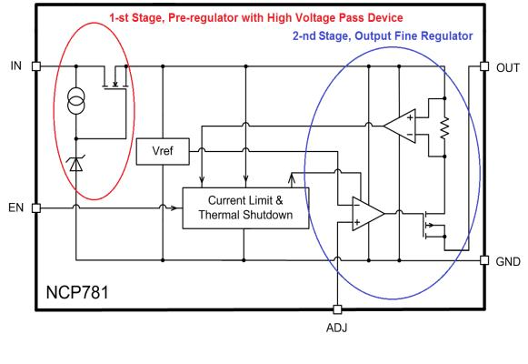
Figure 2. Simplified block diagram
