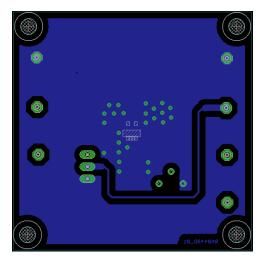
PCB Bottom Side 1874 mm<sup>2</sup> total Cu area, 1815 mm<sup>2</sup> GND Cu area
