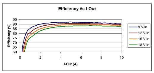
Figure 1: NCP3020 Efficiency at 9V-18.0V with a 3.3V Output Voltage
