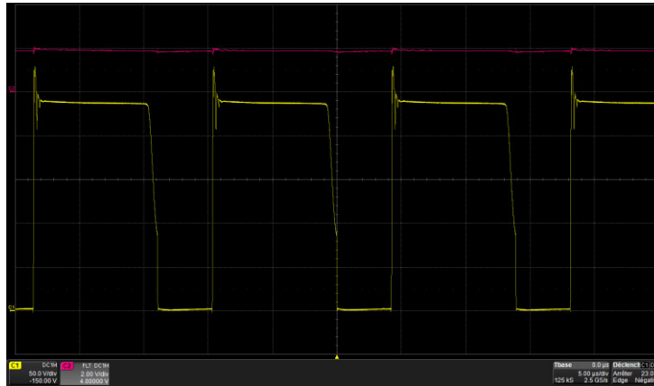
Figure 5. QR (1 st Valley) Operation @ 45 W / 115 V rms
