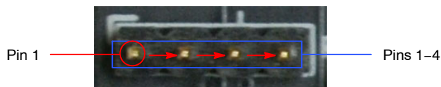
Figure 5. Pin Locations for a Single Jumper. Pin 1 is Located at the Leftmost Side and Increases as it Moves to the Right
