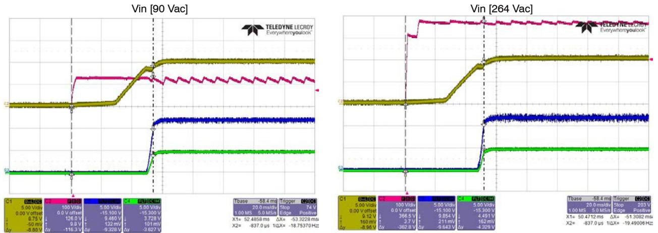
C1 [V<sub>DD</sub>], C2 [V<sub>BULK</sub>], C3 [V<sub>OUT-12V</sub>], C4 [V<sub>OUT-5V</sub>]
