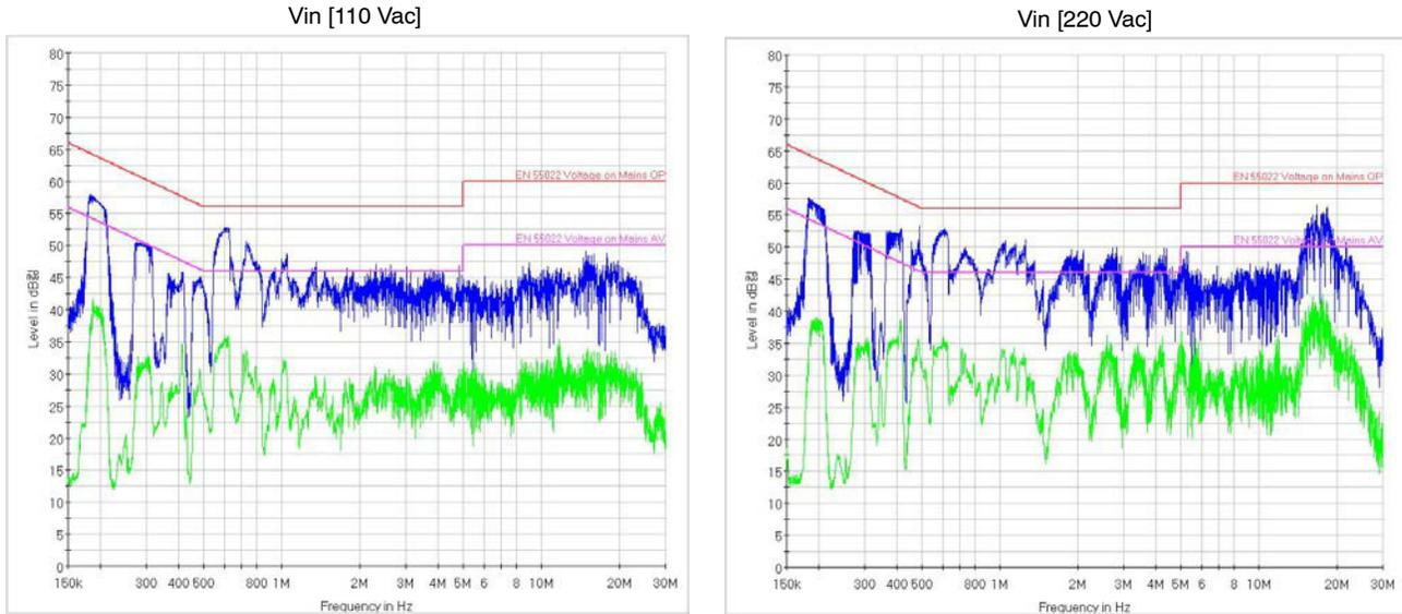
Figure 7. Conducted Emission at Full Load
