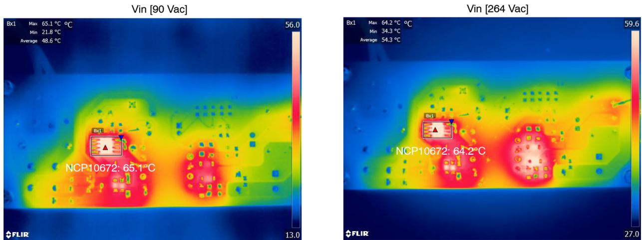
**Figure 10. IC Temperature at Full Load**
