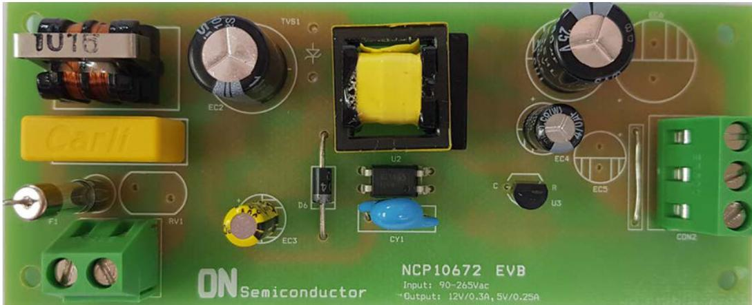
Figure 2. Top Side of Evaluation Board
