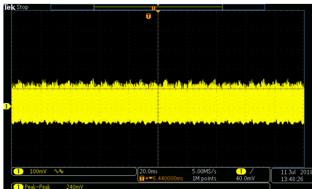
Figure 13. Output Ripple @ 264 Vac Input, 25 A Output
