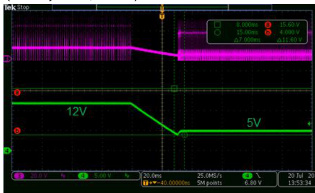
Figure 19. PD Voltage Change from 12 V to 5 V at 0 A
