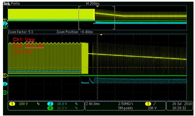
Figure 31. Load Change at 115 Vac and 20 V
