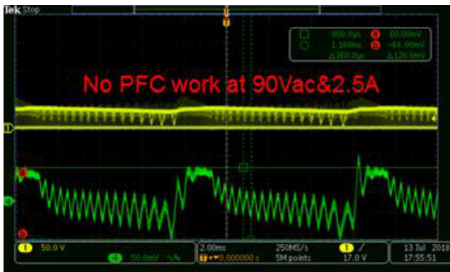
Figure 23. Output Ripple @ 90 Vac and 20 V Output
