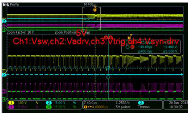
Figure 33. ACF to DCM Mode Transition
