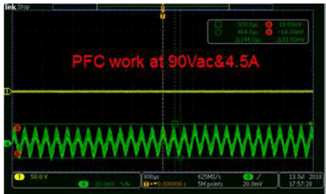
Figure 23. Output Ripple @ 90 Vac and 20 V Output
