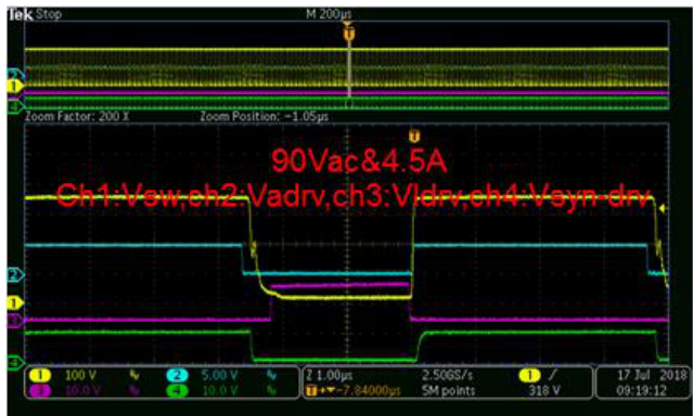
Figure 30. Key ACF Waveform @ 20 V Output
