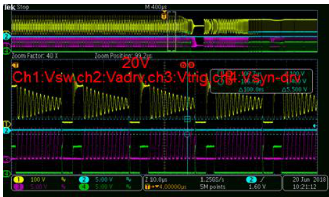
Figure 35. DCM to ACF Mode Transition
