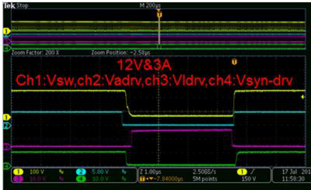
Figure 28. Key ACF Waveform @ 90 Vac Input
