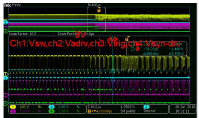
Figure 33. ACF to DCM Mode Transition
