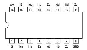
Figure 1. 16-Lead Pinout (Top View)
