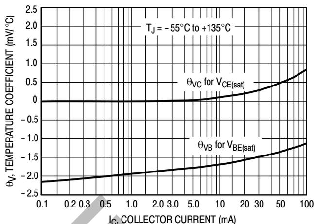
Figure 5. Temperature Coefficients
