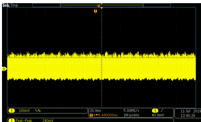
Output Ripple @ 264 Vac Input, 25A Output
