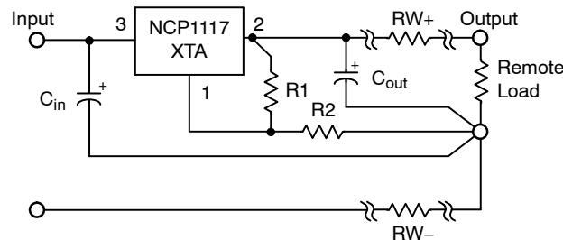
Figure 26. Load Sensing
