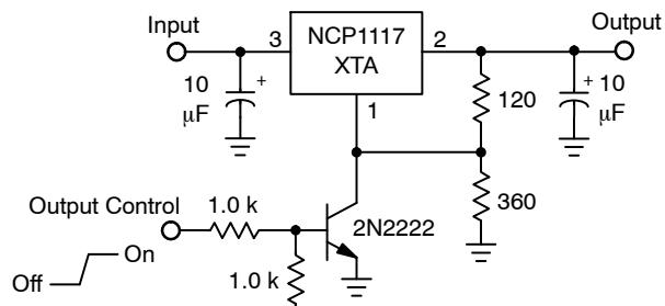
$$V_{out(Off)} = V_{ref}$$
