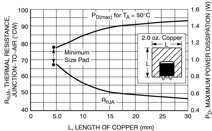
**Figure 22. DPAK Thermal Resistance and Maximum Power Dissipation vs. P.C.B. Copper Length**
