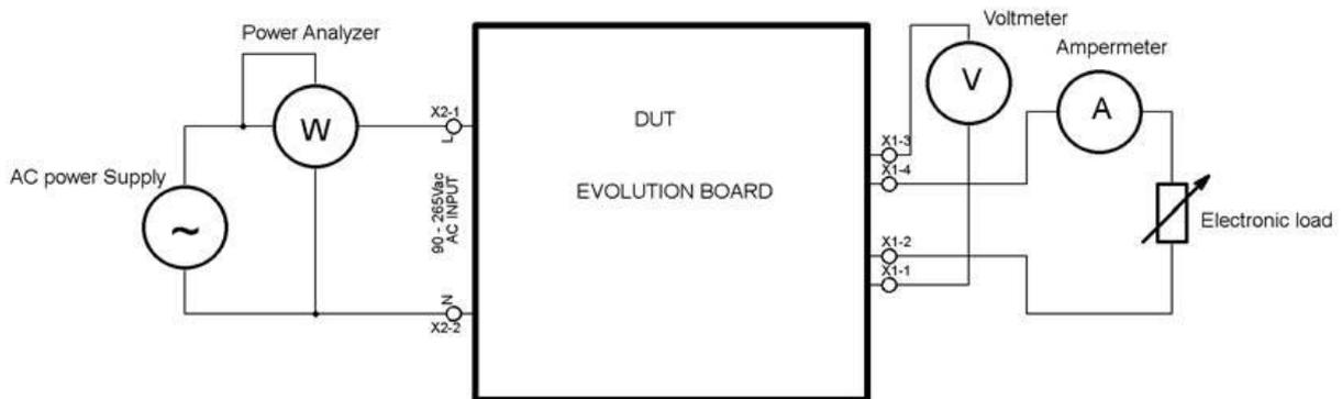
2. Set AC Power Supply to 115 V AC, with current limit approximately 2.5 A – to avoid any unwanted damage. Set Electronic Load to disabled state or to loading current 0 A
