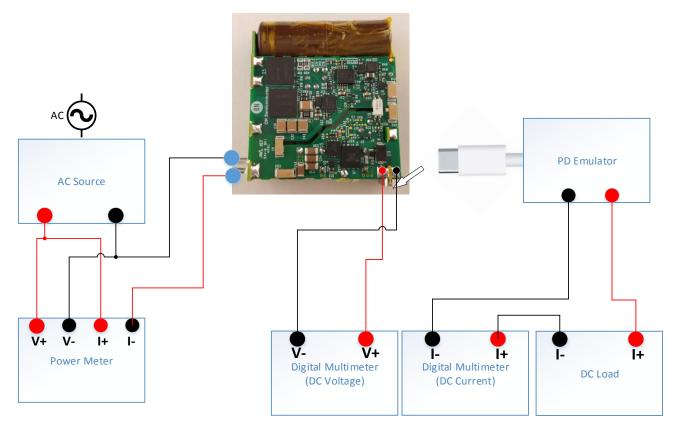
Figure 1 - Test Configuration
