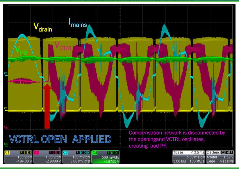
The controller does not stop switching and the FB voltage does not change too much 7/18/2019 VCTRL pin voltage oscillates widely and PF is bad VCTRL Open Before Startup , Vcc=20V is applied Vmains=110 Vac ; Iload=400mA; Vbulk= 390V
