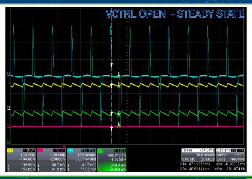
VCTRL gets fully discharged through the compensation resistor
