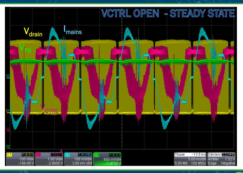
The controller does not stop switching and the FB voltage does not change too much <sup>7/18/2019</sup> VCTRL pin voltage oscillates widely and PF is bad
