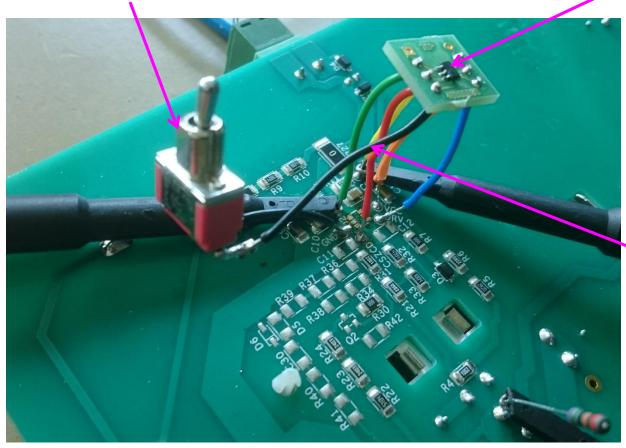
The NCP1602 cannot be directly soldered onto the evaluation board and is sodered onto this TSOP-6 to DIL daughter board which is connected to the Evaluation Board by the colored wires.
