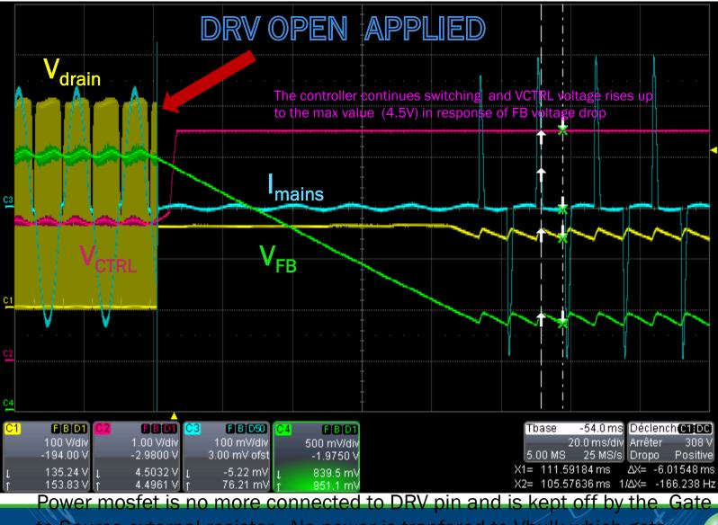
to Source external resistor . No power is tranfered to Vbulk which gets 7/18/2019 discharged by the load current.
