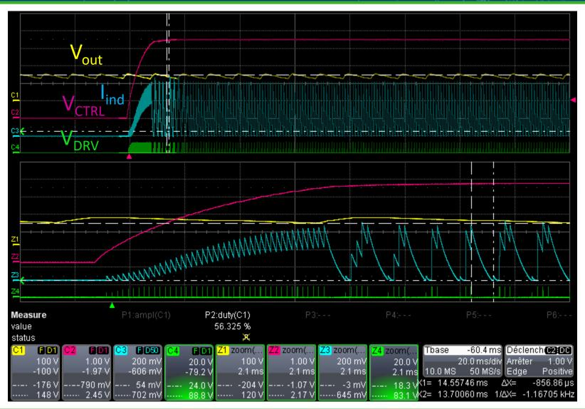
Inductor current is limited to OCP level by OV Semiconductor® system
