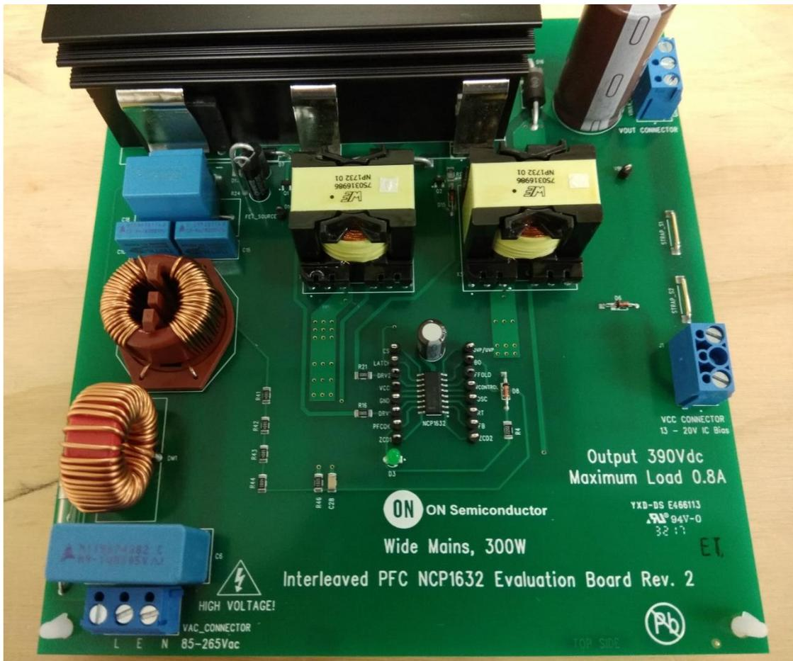
Figure 1 – NCP1632PFCGEVB Evaluation Board
