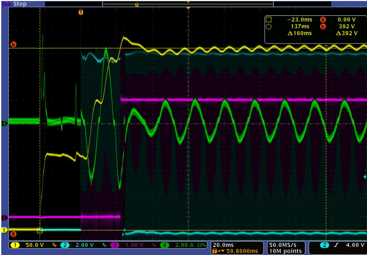
Figure 3 – Start-up waveforms at 115 Vac, 0.3 A load – Vout (Yellow), DRV1 (Blue), Input current (Green) & PFCok signal (Purple)
