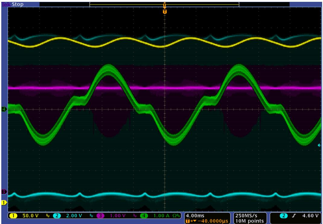
Figure 5 – Input Current (Green) & Vout (Yellow) at 230 Vac, 0.6 A
