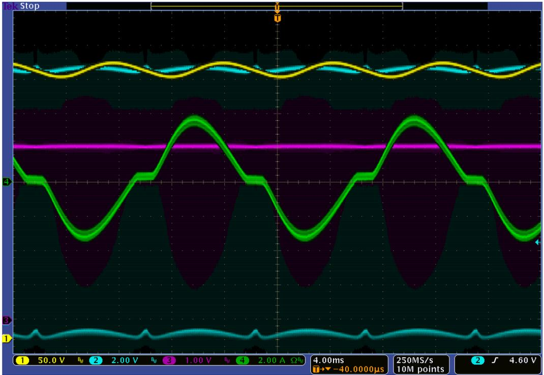
Figure 4 – Input Current (Green) & Vout (Yellow) at 115 Vac, 0.6 A
