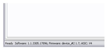
The above figure shows the software version, the board index as being device #2, the firmware version being 1.7 and the NCV53480 silicon version being 4.
