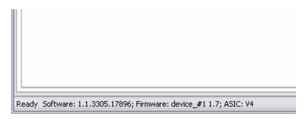
The above figure shows the Software version, the board index as being device #1, the firmware version being 1.7 and the NCV53480 silicon version being 4.
