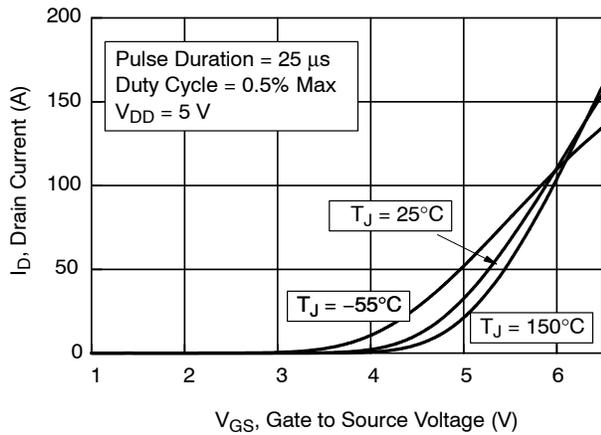
Figure 7. Transfer Characteristic
