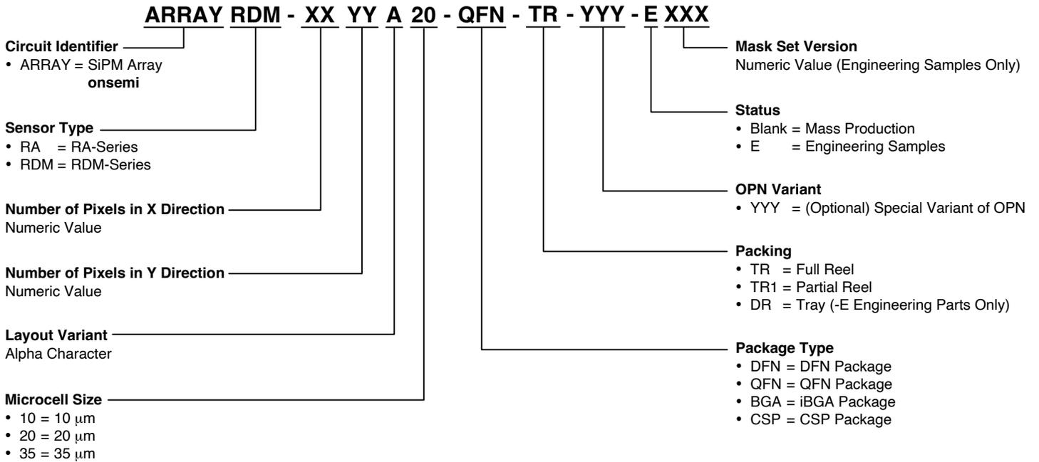
**Naming Convention for LiDAR SPAD Arrays**
