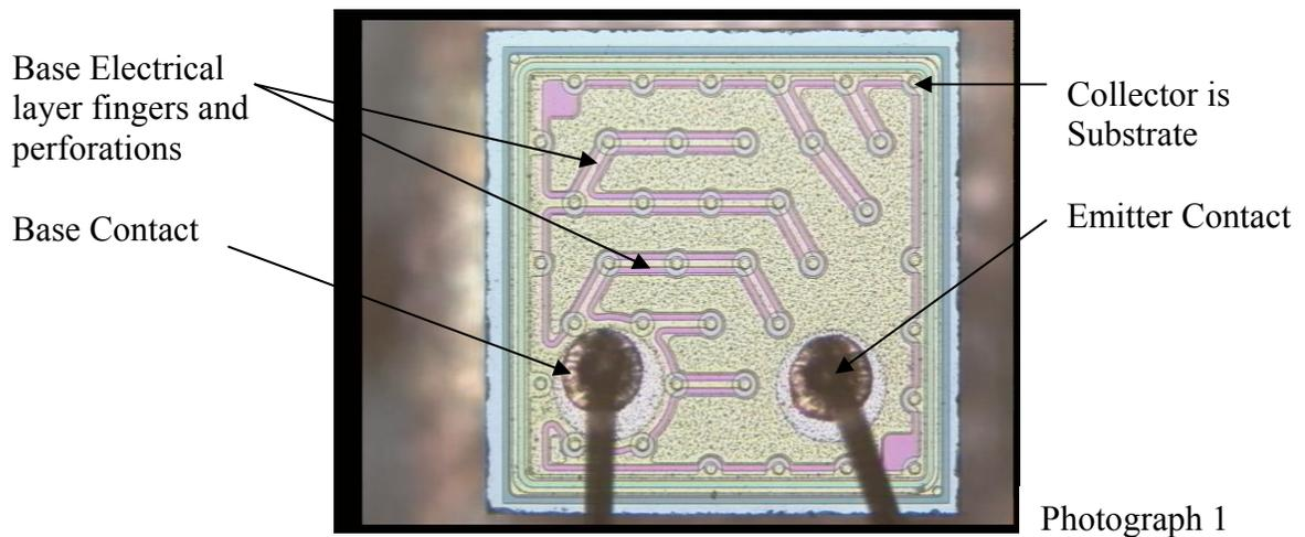
Some of the new Low  $V_{CEsat}$  BJT's are now available with a saturation voltage at 1.0 Amps of well under 50 mV. This equates to a forward resistance of under 50 m $\Omega$ , and proves very competitive against a higher cost MOSFET.
