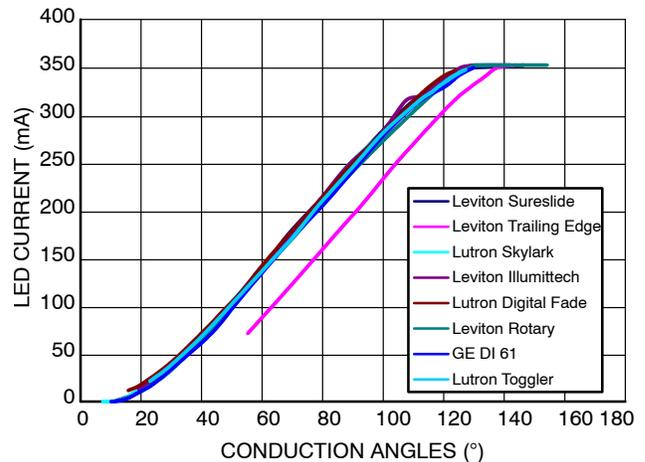
**Figure 6. Dimmer Control Range (Vin = 115 Vac, 12 LED load)**
