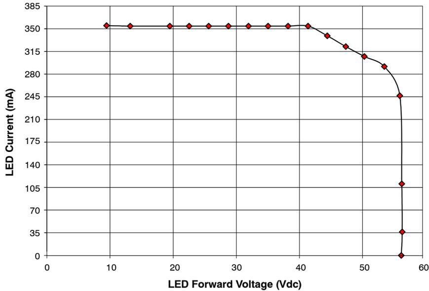
**Figure 5. Current Load Regulation (Vin = 115 Vac)**
