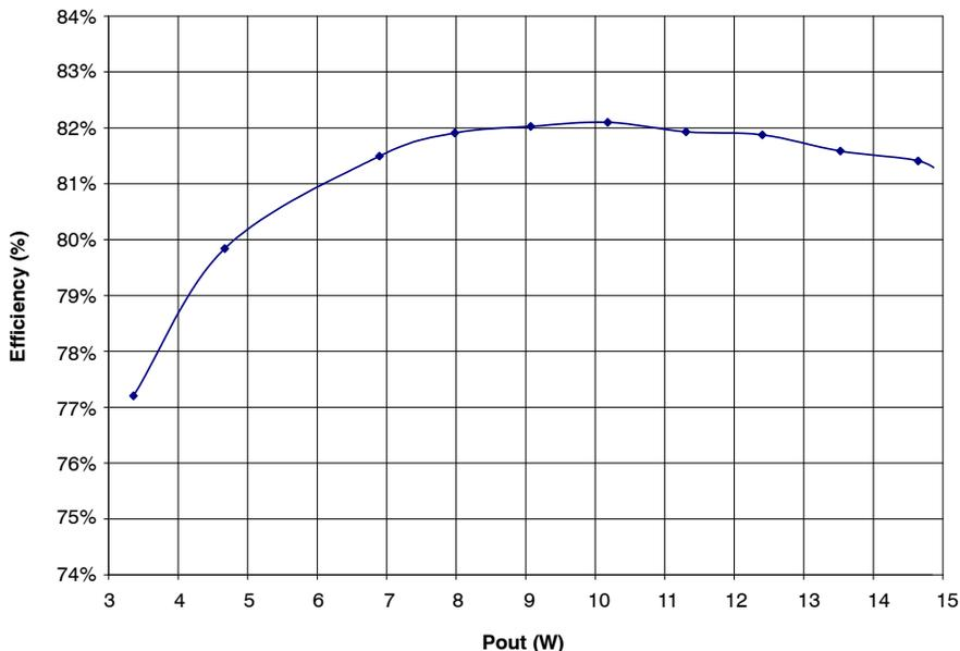
**Figure 4. Efficiency versus load (Vin = 115 Vac)**
