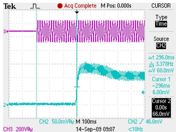
Figure 7. Startup Time ( $V_{in} = 115 \text{ Vac}$ , 12 LED load)
