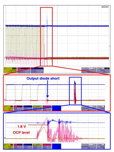
Figure 17. Output Diode Short Protection
