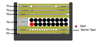
Figure 3. Transformer Winding Structure
