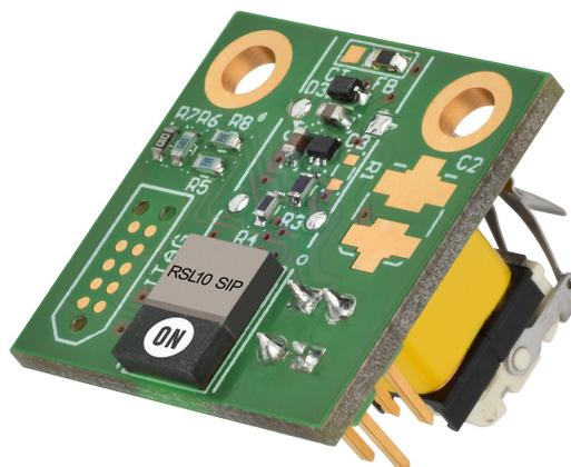
**Figure 2. Energy Harvesting Bluetooth Low Energy Switch**
