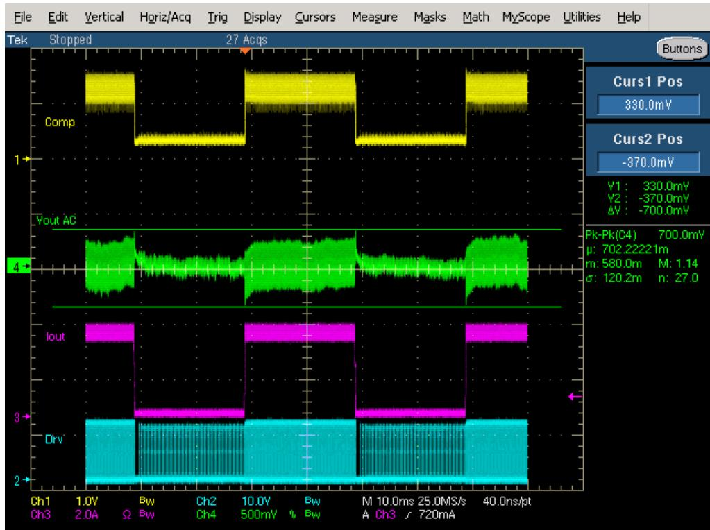
Figure 51. 48 V Input 15 V Output Transient Response
