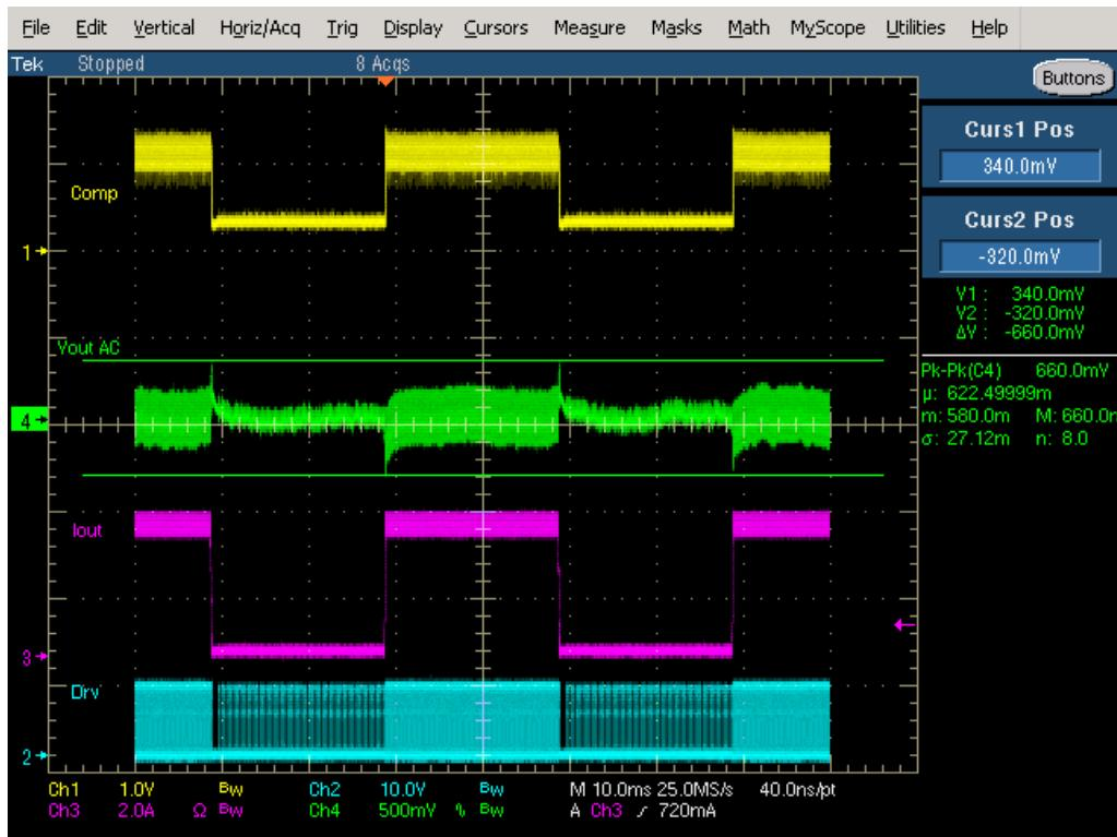
Figure 48. 48 V Input 12 V Output Transient Response
