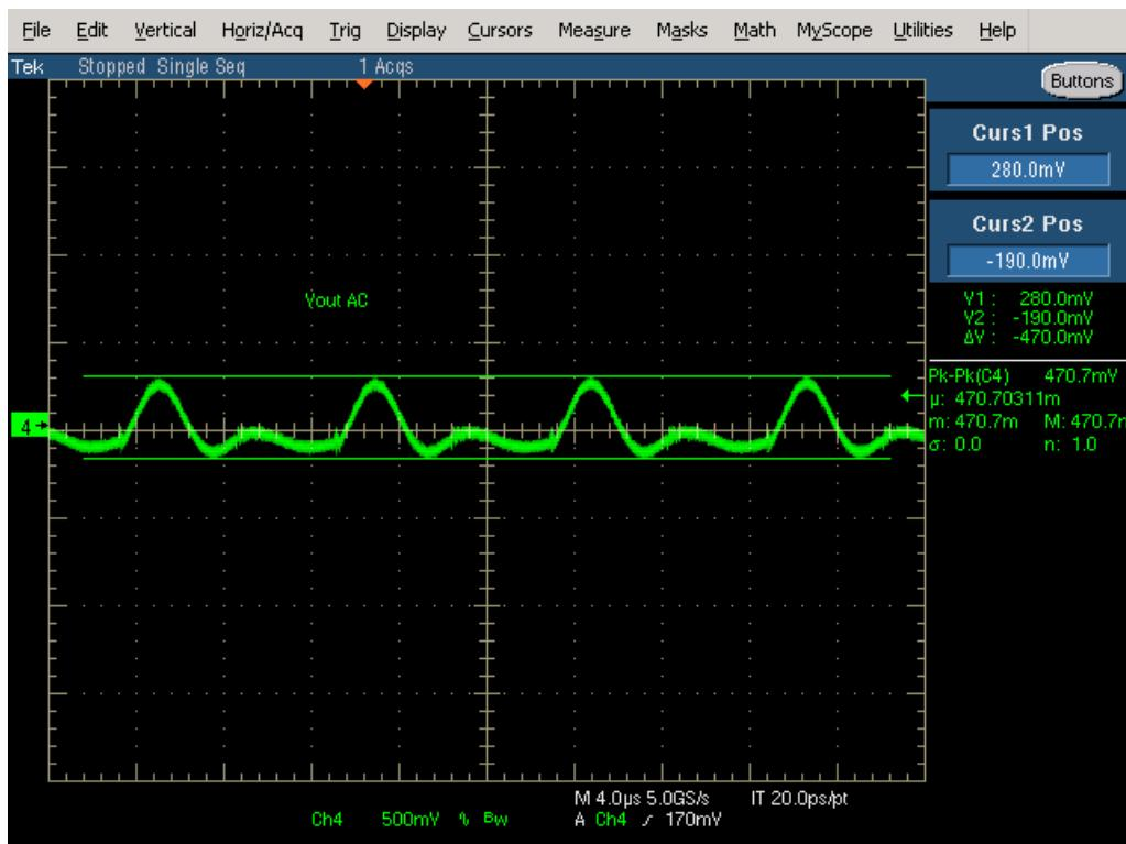
Figure 35. 37 V Input 15 V Output Ripple
