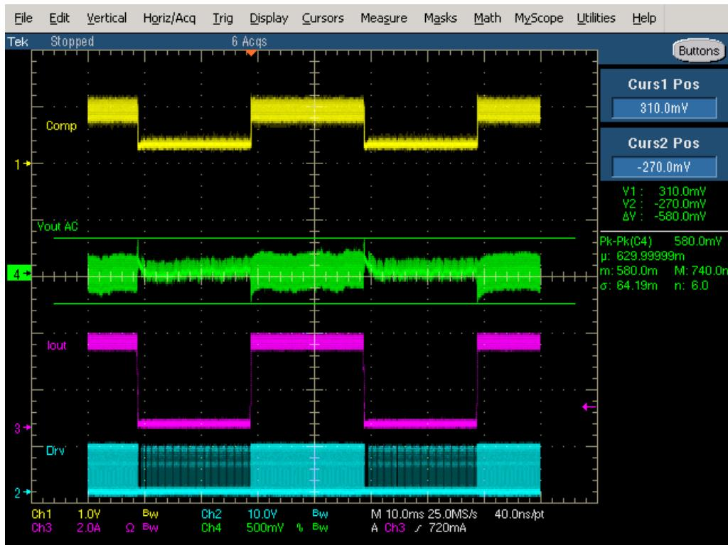
Figure 46. 57 V Input 9 V Output Transient Response
