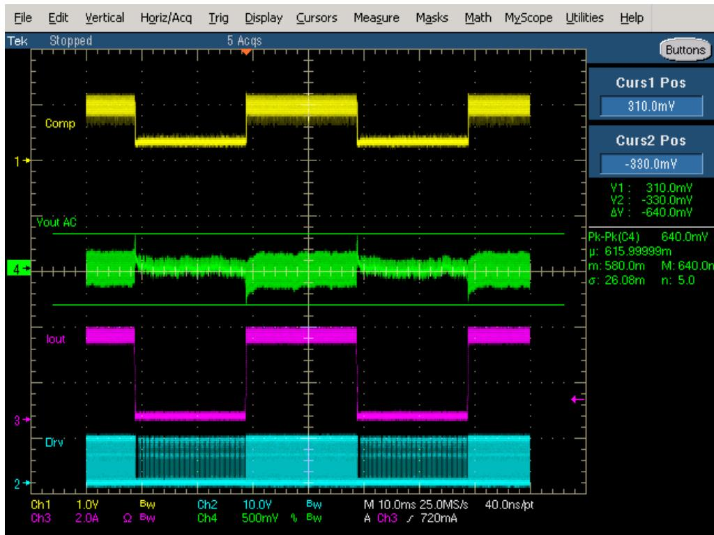
Figure 44. 37 V Input 9 V Output Transient Response
