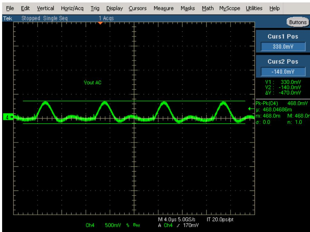
Figure 37. 57 V Input 15 V Output Ripple
