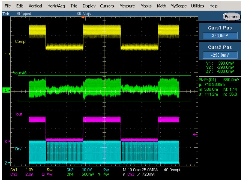
Figure 54. 48 V Input 20 V Output Transient Response
