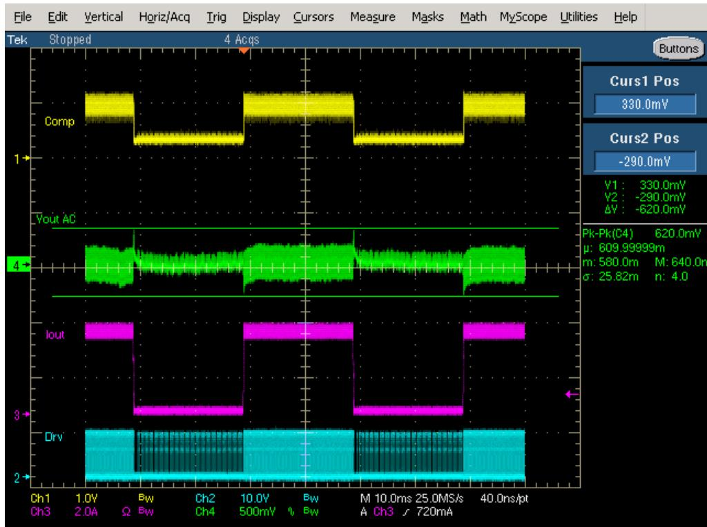
Figure 45. 48 V Input 9 V Output Transient Response
