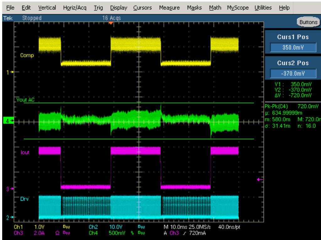
Figure 49. 57 V Input 12 V Output Transient Response
