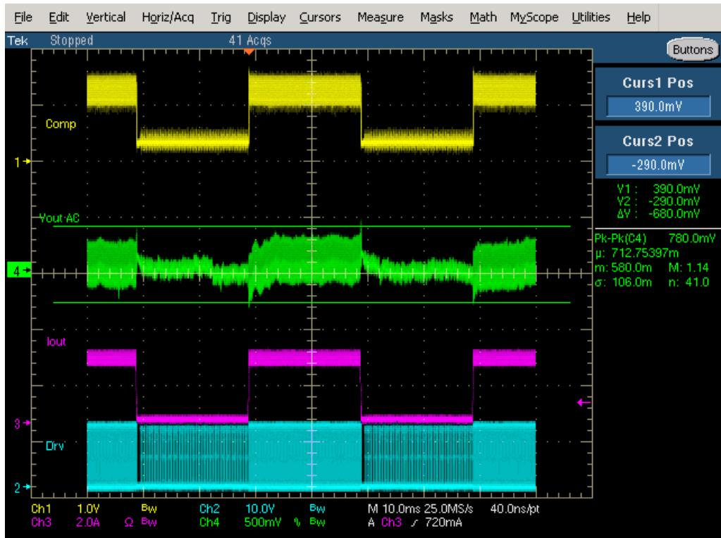
Figure 55. 57 V Input 20 V Output Transient Response
