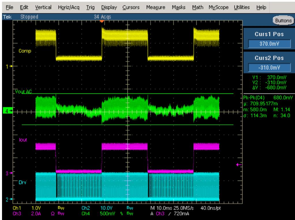
Figure 53. 37 V Input 20 V Output Transient Response
