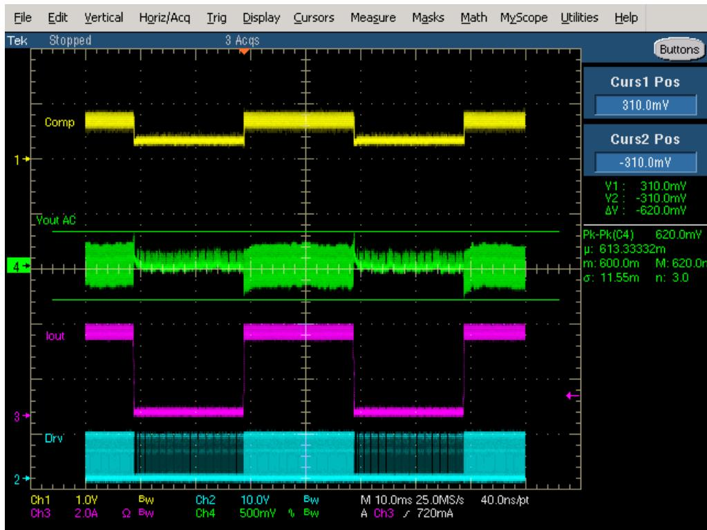
Figure 42. 48 V Input 5 V Output Transient Response
