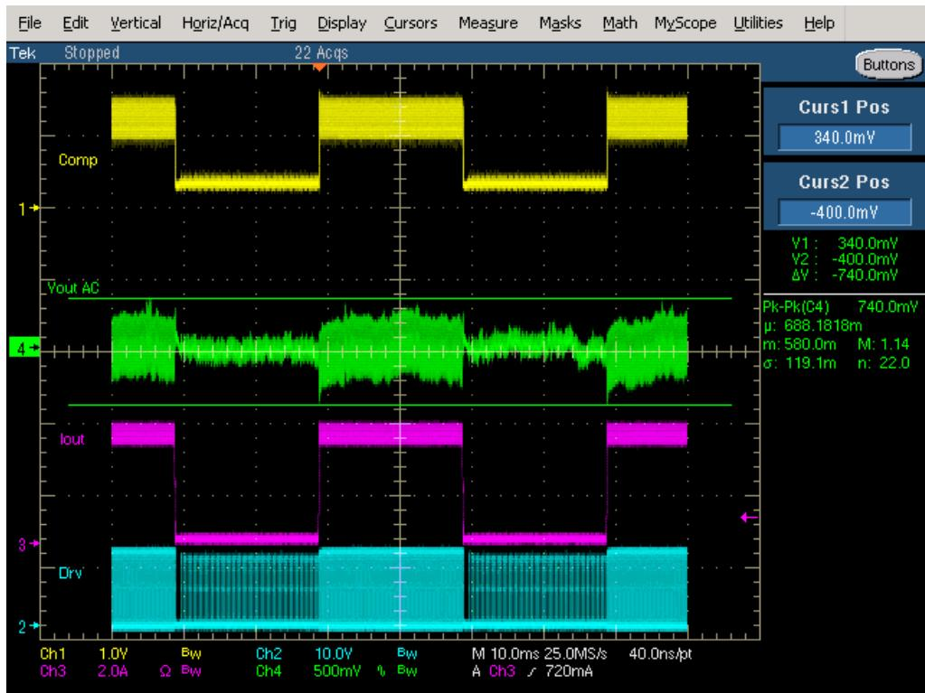
Figure 52. 57 V Input 15 V Output Transient Response
