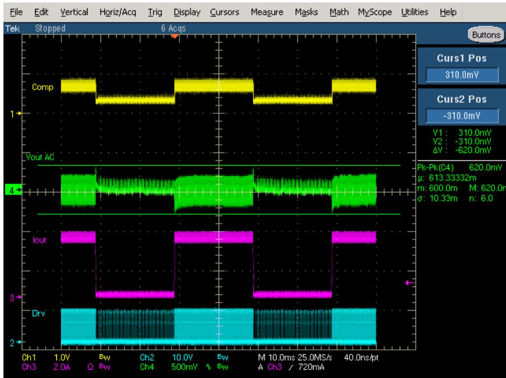
Figure 43. 57 V Input 5 V Output Transient Response
