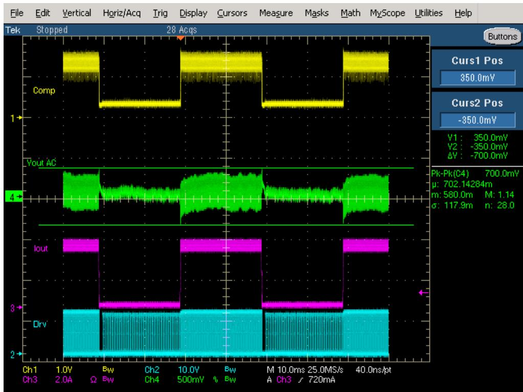
Figure 50. 37 V Input 15 V Output Transient Response
