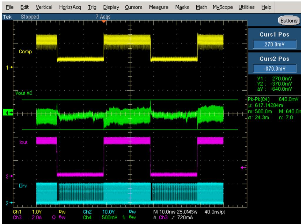
Figure 47. 37 V Input 12 V Output Transient Response
