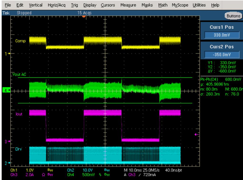
Figure 41. 37 V Input 5 V Output Transient Response
