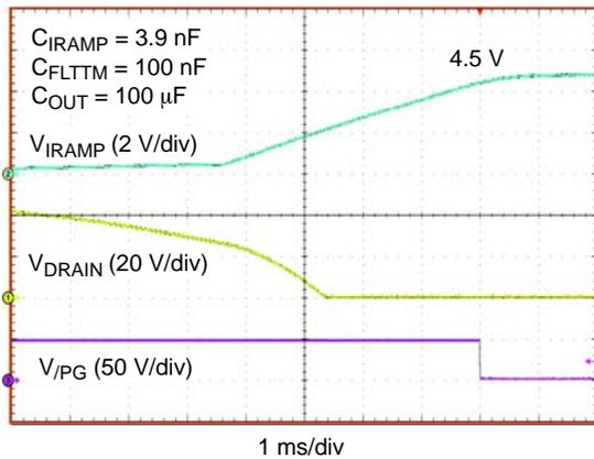
**Figure 13.  $\overline{\text{PG}}$  Output Timing - Current Qualified**
