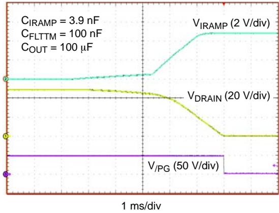
**Figure 12.  $\overline{\text{PG}}$  Output Timing - Voltage Qualified**
