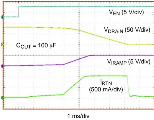
Figure 5. Start-up from Enable,  $V_{IN} = -80\text{ V}$
