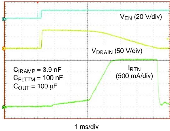
Figure 4. Live Insertion Event,  $V_{IN} = -80\text{ V}$
