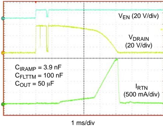
Figure 3. Live Insertion Event,  $V_{IN} = -48\text{ V}$
