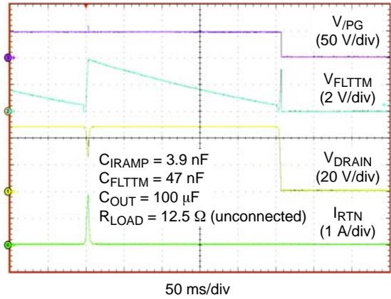
**Figure 10. Recovery from a Fault (TPS2399 only)**
