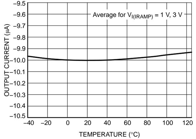
Figure 18. IRAMP Output Current – Fast Rate
