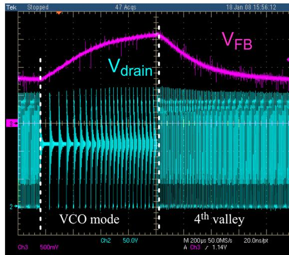
Figure 6. The Controller Hesitates Between VCO Mode and 4<sup>th</sup> Valley:  $C_t$  is Too Big!
