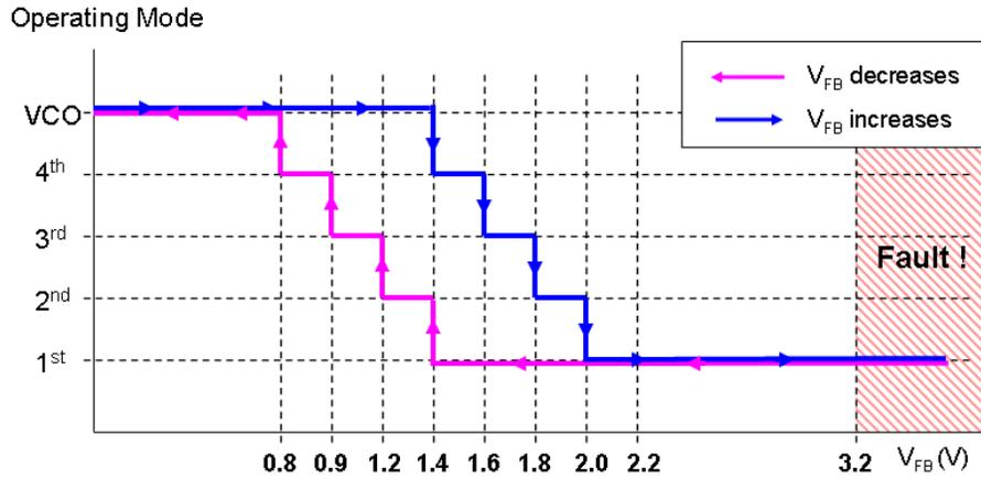
**Figure 3. Operating Valley According to FB Voltage**
