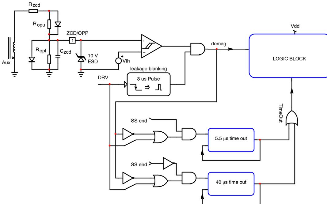
Figure 8. Zero-Crossing Detection Bloc Schematic
