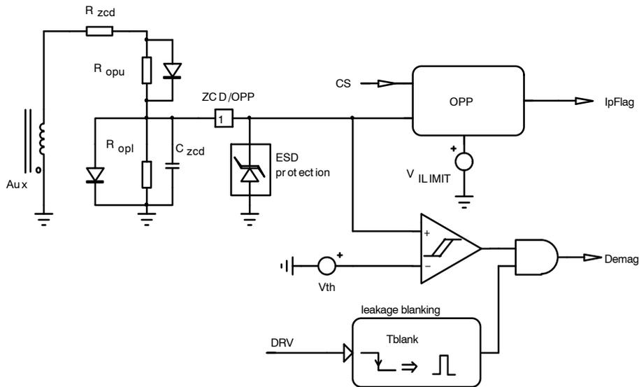
**Figure 9. ZCD and OPP Circuit**
