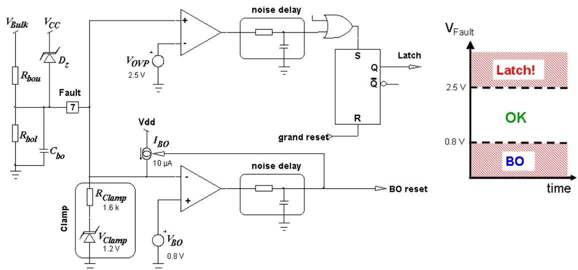
Figure 13. BO / OVP Combination in NCP1379, NCP1380 C and D Versions
