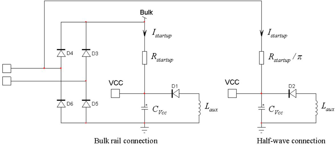
**Figure 10. The Startup Resistor can be Connected to the Bulk Rail or to the Half Wave**
