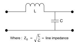
Figure 1. Lossless Transmission Line – Equivalent Circuit
