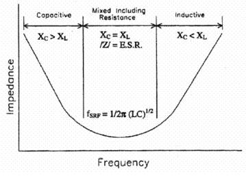
Figure 3. Impedance vs. Frequency Characteristic for a Capacitor
