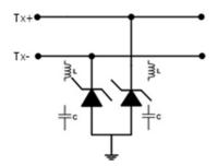
Figure 2. ESD Protection Device – Parasitic Model
