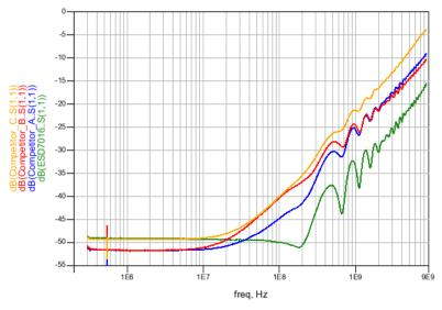
Figure 7. Return Loss (S<sub>11</sub>) Characteristics of USB 3.0 ESD Protection Devices
