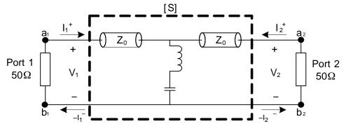
Figure 5. Two Port Electrical Network of Lossless Transmission Line
