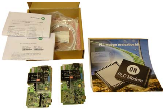
Figure 1. Contents of a PLC Evaluation Kit
