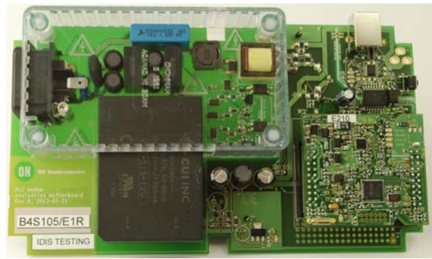
Figure 2. Evaluation Board: Motherboard and Plugged-on Daughterboard
