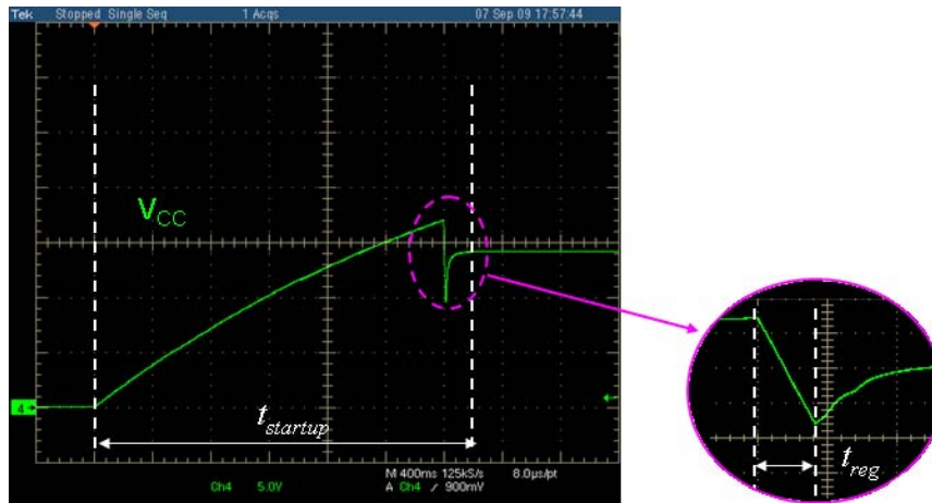
Figure 8. V CC Waveform during Startup
