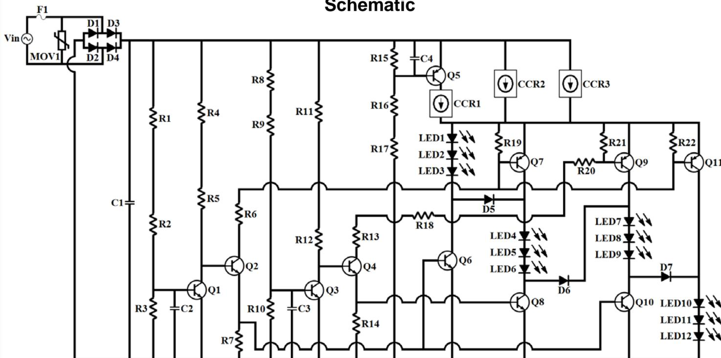
Figure 1: Three-Stage 230 Vac CCR lighting circuit
