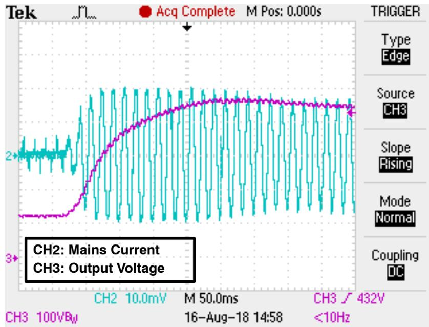
Figure 9. 90 V ac Full Load Startup
