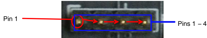
Figure 5. Pin Locations for a Single Jumper. Pin 1 is Located at the Leftmost Side and Increases as it Moves to the Right
