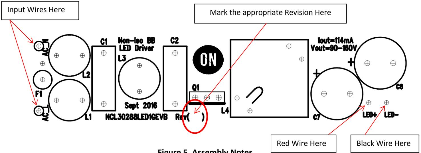
1. Strip and tin lead wires to 6" ± 0.5" 4 Places. Red for LED+, Black for LED-, White for AC\_L and AC\_N
