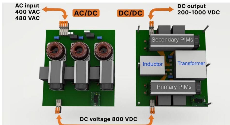
Figure 1. 25 kW DC Fast Charger Reference Design (Left – PFC Stage, Right – Dual Active Bridge)
