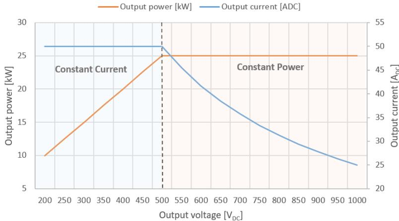
Figure 3. Power and Current Profile of the 25-kW DC Charger Power Stage. The Current is Limited to 50 A Below 500 V.
