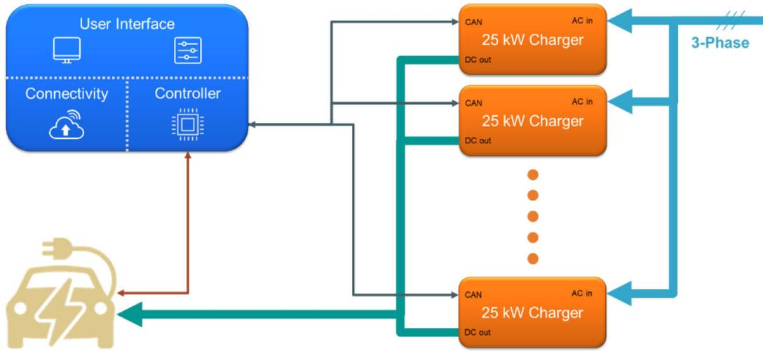
Figure 2. Overview of the Main Blocks in a DC Fast Charger
