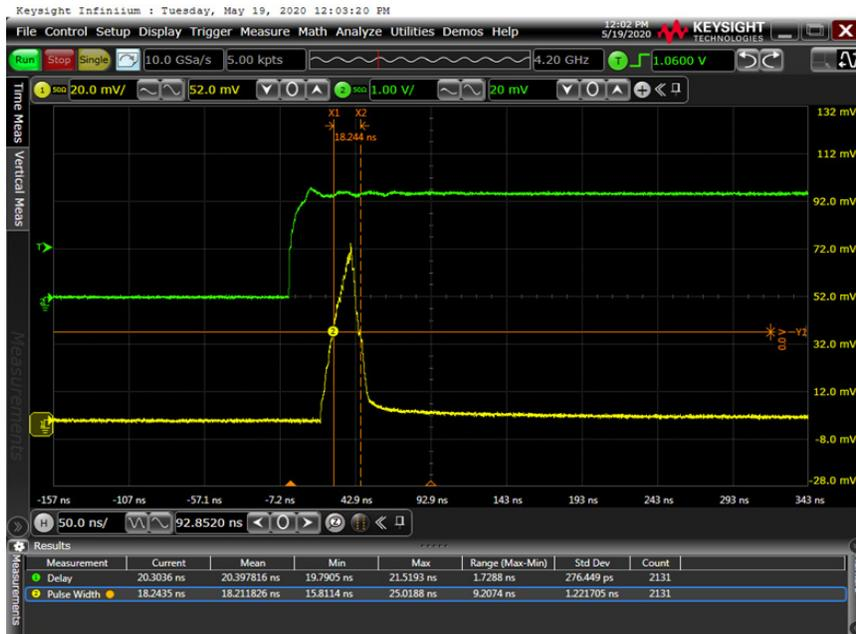
Figure 40. Typical Laser Optical Pulse Shape
