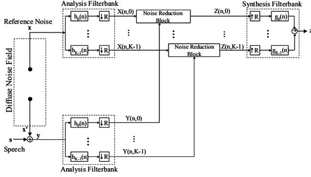
Fig. 1. Block diagram of the SAF system.
