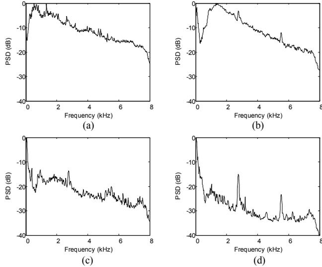
**Fig. 3. Power Spectral Density (PSD) of the noises recorded by two microphones in various situations: (a) Sit-MallI, (b) HWY, (c) CarWOpen, (d) CarWClose.**
