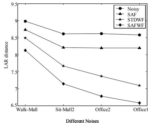
Fig. 7. LAR-distances for the noisy inputs and the outputs of the SAF, STDWF and SAFWF techniques in four new recording environments.
