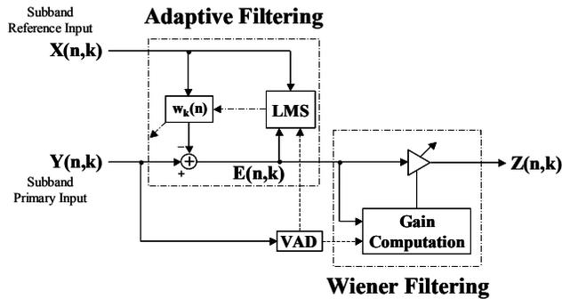
Fig. 2. Block diagram of the noise reduction block.
