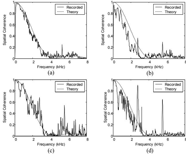
**Fig. 4. Spatial coherence of the noises recorded by two microphones in various situations: (a) Sit-MallI, (b) HWY, (c) CarWOpen, (d) CarWClose.**
