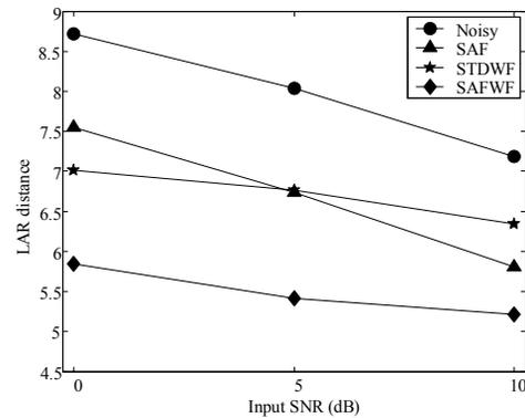
Fig. 6. LAR-distances for the noisy inputs and the outputs of the SAF, STDWF and SAFWF techniques for CarWClose case and different input SNRs.
